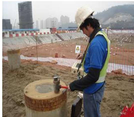
The PIT, is a low strain testing method which is used to quickly perform quality control tests of a large number of piles. The impact produces a compression wave which travels down the pile at a constant wave speed. Changes in cross sectional area, such as a reduction in diameter, or material - such as a void in concrete, produce wave reflection.
